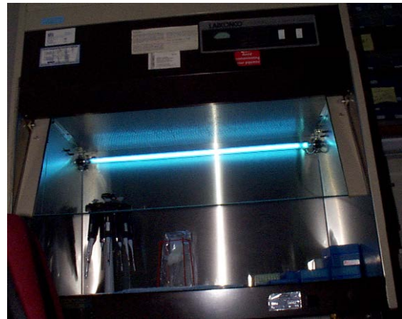
Figure 1. Biosafety cabinet with operating UV germicidal lamp. Direct and reflected exposures can be hazardous.
